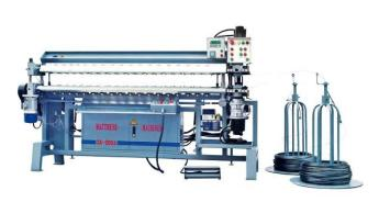
**SX100** can be used for mass production of springs, or can work in tandem with an assembling machine **SX200S** for production of mattress spring frames.
